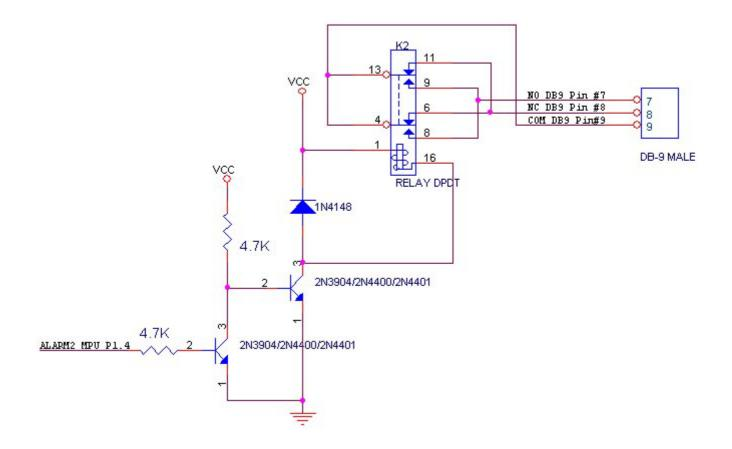
Figure 62: Hard Alarm Output Relay
