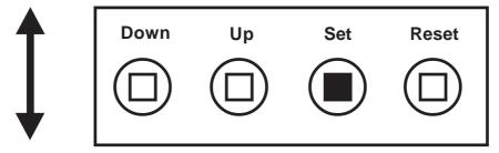
Figure 5: Four Front Pannel Push Buttons of Portable Speed DVR System (Set)
