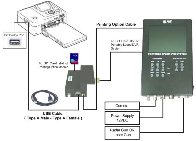
Figure 78: Connection Diagram between Printing Option Module and Portable Speed DVR System
